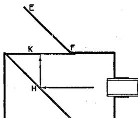
in the opposite end of the box. This reflects the rays of light passing through the lens to the surface K, which may be either of ground or plain glass. The lid or cover EF protects the glass and keeps the strong light out when sketching. The inside of the box and brass tube are painted a dull black.
