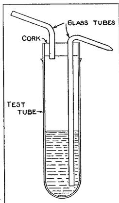
of the test tube and the other just projecting through the cork. The spray tube may be made with a fine hole by first securing a tube longer than necessary and heating it at the proper point and drawing the tube out into a fine thread. The thread is broken off at the
