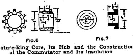
Fig. 6 Armature-Ring Core, Its Hub and the Construction of the Commutator and Its Insulation
