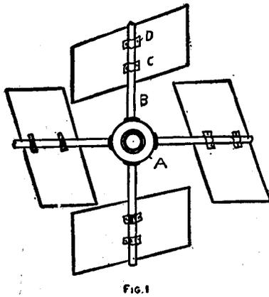
blades should be of sheet metal or thin hardwood. The sizes may vary according to the capacity of the wheel and amount of room for the blades on the spokes. Each one is tilted so as to receive the force of the wind at an angle, which adjustment causes the wheel to revolve when the wind pressure is
