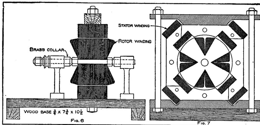
about 2-1/2 lb. being used, and the connections are such as to produce alternate poles--that is, the end of the first coil is joined to the end of the second the beginning of the second to the beginning of the third, and the end of the third to the end of the fourth, while the beginnings
