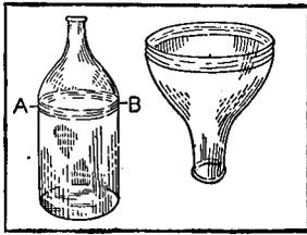
Secure a glass bottle having a small neck and tie a string saturated in kerosene around the outside at A and B as shown in the sketch. Light the string and allow it to burn until the glass is heated, then plunge the bottle quickly into water. The top or neck will then come off easily. The sharp edges are ground or filed off smooth. This will make a good emergency funnel which serves the purpose well for filling wide necked bottles.-
