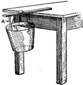
between the end of the stick on the table and the bottom of the pail. This makes the center of gravity somewhere near the middle of the stick on the table, thus holding the pail as shown.
