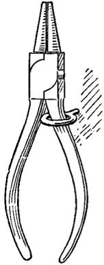
by placing rows of different-size screw eyes on a wall close to the workbench, so that files, chisels, pliers and other tools, and the handles of hammers can be slipped through the eyes.
