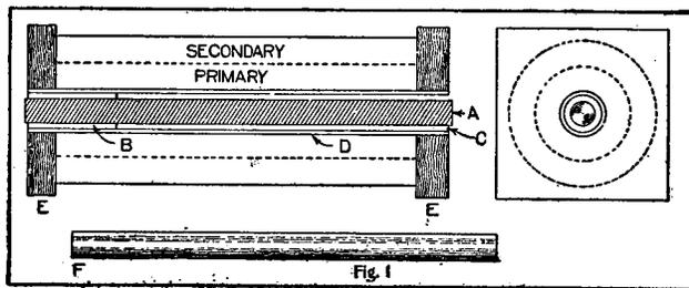
paper and coming in contact with the layer beneath, thus causing a short circuit. The secondary winding should have at least a dozen layers and should be carefully wound to prevent short circuiting.
