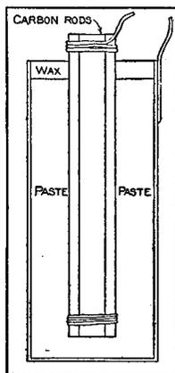
A cell of this kind can easily be made, and to make it the proper size a sheet of zinc 8-1/2 in. long and 6 in. wide will be required. This zinc is rolled into a cylinder 2-1/2-in. in diameter. This will allow for a lap of 5/8 in., which is tightly soldered only on the outside of the seam. Close one end of the cylinder by soldering a disk of zinc over it, making a
