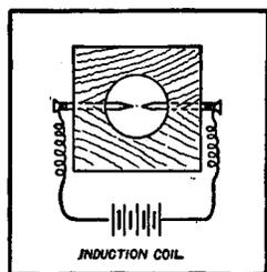
or the circuit closed in some other way the discharge occurs. The distance between the nail points--which must be bright and clean--should be just enough to give a good, fat spark. --Contributed by Geo. W. Fry, San Jose, Cal.
