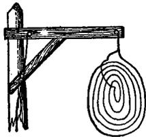
good contact for the sliding piece. The tuning is done by sliding the contact piece, which is made of light copper wire, along the convolutions of the tuning coil until you can hear the signals. The signals are heard in a telephone receiver, which is shown connected in shunt across the binding posts of the lamp holder with one or two cells of dry battery in circuit, Fig. 7.
