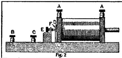
will be almost unnoticeable, but when it is withdrawn the current will be so strong that a person cannot let go the handles until the coil is shut off. After the secondary coil is wound it should be covered with stiff paper, and the whole coil, including the wood ends, should then be enameled black.
