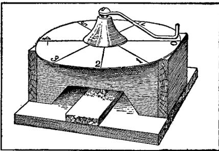
and the construction is complete. The base is improved for the measuring work by fastening a small piece of wood on the board between the legs of the bench. A small piece of metal is glued on this piece of wood at the point where the bolt meets it.
