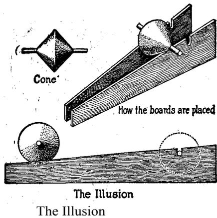
one end will be higher than the other by a little less than half the diameter of the cone. Thus it will be seen that the diameter of the cone determines the length of the slope of the tracks. A notch should be cut in the tracks, as indicated, for the shaft to drop into at the end of the course.
