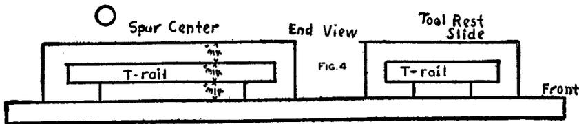
with screws, two more pieces 7 by 3/4 by 3/4 in., Fig. 5, B. This tail-piece should move smoothly back and forth with no side motion. Now get a block of hardwood 4 by 2-1/4 in., and 1-3/4 in. higher than the spur center when mounted on the middle of the tail-piece just described. At exactly the height of the spur center bore through this block a 3/4-in. hole, Fig. 5. Have
