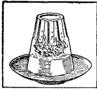
Place a small piece of paper, lighted, in an ordinary water glass. While the paper is burning turn the glass over and set into a saucer previously filled with water. The water will rapidly rise in the glass, as shown in the sketch.
