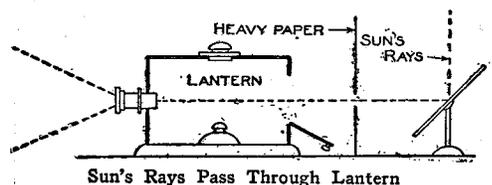
cut in the paper and the lantern placed on a table in front of the hole, the lamp having been removed and the back opened. The lantern must be arranged so that the lens will be on a horizontal line with the hole in the paper. A mirror is then placed just outside of the window and at such an angle that the beam of light is thrown through the hole in the paper and the lens of the lantern.
