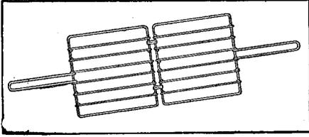
as the other wires. This will leave the handle laying across the other side of the frame. The frame is fastened to the handle on this side by giving the handle one turn around the frame. The inside edges of the frame are now tied together with a small ring of wire which is loose enough to allow each half to swing freely. --C. D. M.
