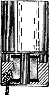
lamp cord, passed through a hole in the bottom of the can and knotted inside to prevent pulling out.
