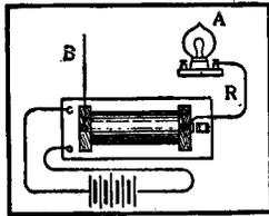
Take a jump-spark coil and connect it up with a battery and start the vibrator. Then take one outlet wire, R, and connect to one side of a 2-cp. electric lamp, and the other outlet wire, B, hold in one hand, and press all fingers of the other hand on globe at point A. A bright, blue light will come from the wires in the lamp to the surface of the globe where the fingers touch. No shock will be perceptible.
