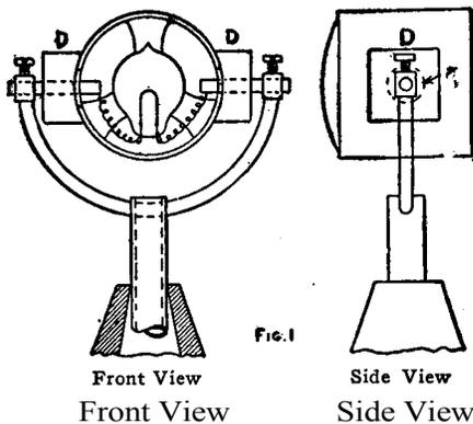
Make two rings of brass wire to fit tightly into the cylinder, trace a circle (inside diameter of cylinder) on a piece of cardboard; place cardboard on glass and cut out glass with a glass cutter; break off odd corners with notches on cutters and grind the edge of the glass on an ordinary red brick using plenty of water. Place one brass ring in cylinder, then the glass disc and then the other ring.
