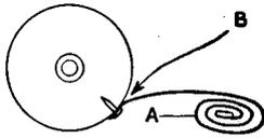
and while in this position apply an ample quantity of glue near the tacks, as shown at B. A shade attached in this manner will not come loose from the roller.
