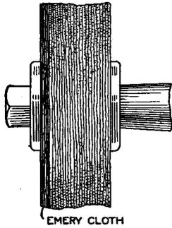
The work of finishing a number of brass castings with flat sides was accomplished on an ordinary polishing wheel, from which the first few layers of cloth were removed and replaced with emery cloth. The emery surface of the cloth was placed outward and trimmed to the same diameter as the wheel. This made a sanding and polishing wheel in one. --Contributed by Chester L. Cobb, Portland, Maine.
