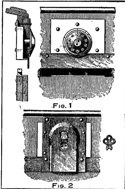
A small combination lock for chests can be purchased for a small sum of money and attached to a trunk cover after first removing the old lock as shown in Fig. 1. It is necessary to add 1/2-in. to the thickness of the trunk lid or cover. This may be done by placing a brass plate 1/8-in. thick on the outside and a board 3/8-in. thick on the inside. The lock, brass plate, board and trunk cover are all securely riveted together. The support for the dial is soldered to the brass plate.
