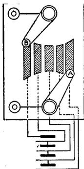
direction to the desired strength. In the various positions of these two switches the current from each individual cell, or from any adjacent pair of cells, may be used in either direction. --Contributed by Harold S. Morton, Minneapolis.
