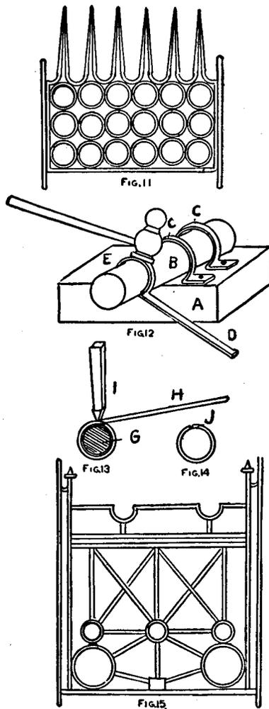
sufficiently stiff by uniting two sides with rivets. The ends at top are looped as shown, while the ends or butts at the base are opened out to make the feet. Rings are shaped on forms and are then riveted to the base cross-piece as illustrated. Crosses are made to describe central design and the plan is worked out quite readily with the different shapes.
