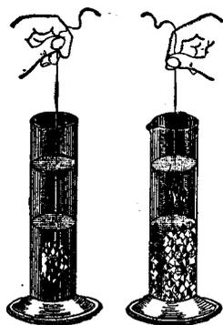
the extremity of which is fixed a small crystal of hyposulphite of soda. The crystal traverses the solution of acetate without causing trouble, but crystallization will immediately set in as soon as it touches the lower hyposulphite of soda solution, as shown at the left in the sketch.
