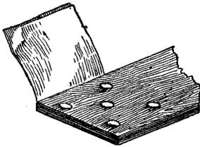
The rubbing of the hot iron over this cloth absorbs just enough of the wax to make the iron work smoothly. When the supply of wax is exhausted, it can be easily renewed. -- Contributed by A. A. Houghton, Northville, Mich.
