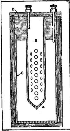
as possible, except for about 1 in. on each end. One end of this tube is hammered together as shown at A in the sketch to make a pocket to hold the paste. This, of course, does not need to be watertight.
