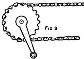
the roof line as at B, then put in the cross-pieces, G G. Seats, E E, are simply boxes. The drive of the car is effected by using the driving sprockets, D D, fitted to the crosspieces, G G, with the original bearings. The parts are thereby secured to the car and the chain placed on.
