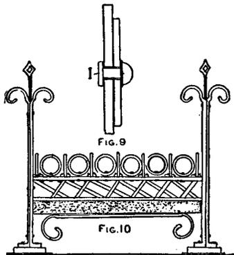
for making these stands, as every part is bent as described in connection with the bending forms, and the portions are simply riveted at the different junctures. Both iron and copper rivets are used as at I, in Fig. 9, a cross sectional view.
