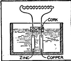
from these ends and they are run through a piece of cork. Attach to the wires, on the under side of the cork, a piece of zinc to one end and a piece of copper to the other. The cork is then floated on a solution of acid, with the zinc and copper hanging in the solution. If zinc and copper are used, the solution is made from water and blue vitriol. If zinc and carbon are used, the solution is made from sal ammoniac and water.
