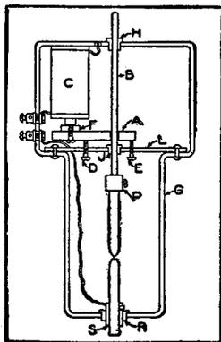
the top and 4 in. at the bottom. A cross bar, L, made of the same material, is fitted into the off-set in the frame and riveted. Holes are drilled through the frame and brass bushings, H and J, are fitted for bearings to receive the adjusting brass rod, B, which should be  $\frac{1}{4}$  in. in diameter. A brass curtain rod can be used for the rod B, and on its lower end a socket, P, is soldered.
