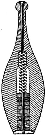
An ordinary Indian club can be fixed so that different weights may be had without changing clubs. Each club is bored to receive lead washers which are held in place by a spiral spring. A bolt is run through from the handle end and fastened with a round nut. The lead washers and spring slip over the bolt as shown in the illustration. Changing the number of washers changes the weight of the club. --Contributed by Walter W. White, Denver, Colo.
