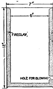
diameter is 7 in., and then rivet the seam. Fit in a round piece of sheet iron for the bottom. Make a hole about the size of a shilling in the side, 2 in. from the bottom. This is for blowing.
